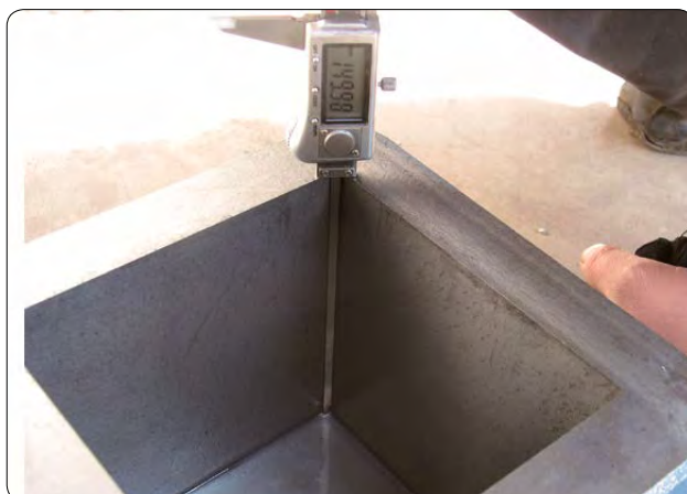
Verification of dimension using electronic digital display depth caliper
