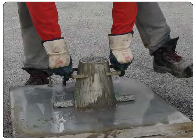
The upside down funnel filled with concrete prior to lifting.
