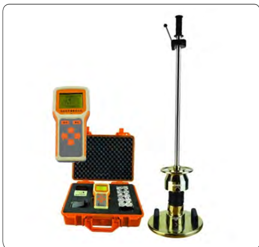
EVD Light-weight falling weight deflectometer
