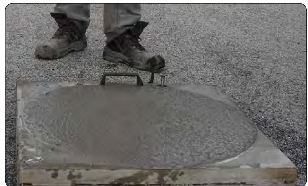
The diameter of the resulting flow is measured. These images show a flow test with very fluid concrete for a special application which made compression impossible.
