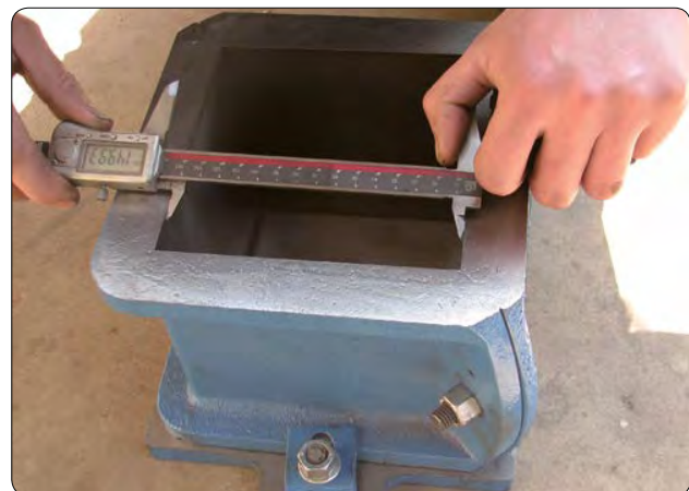
Verification of dimension using digital vernier caliper
